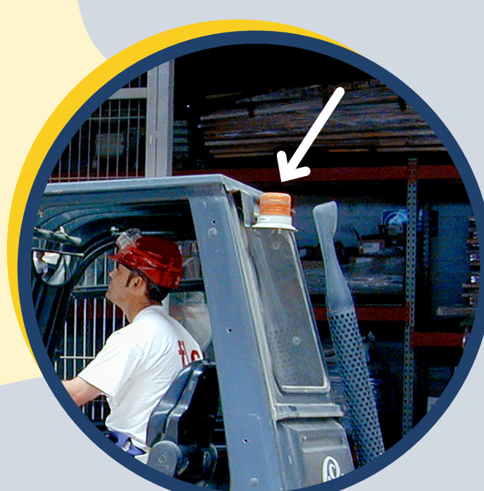
Detail of a forklift truck light .
